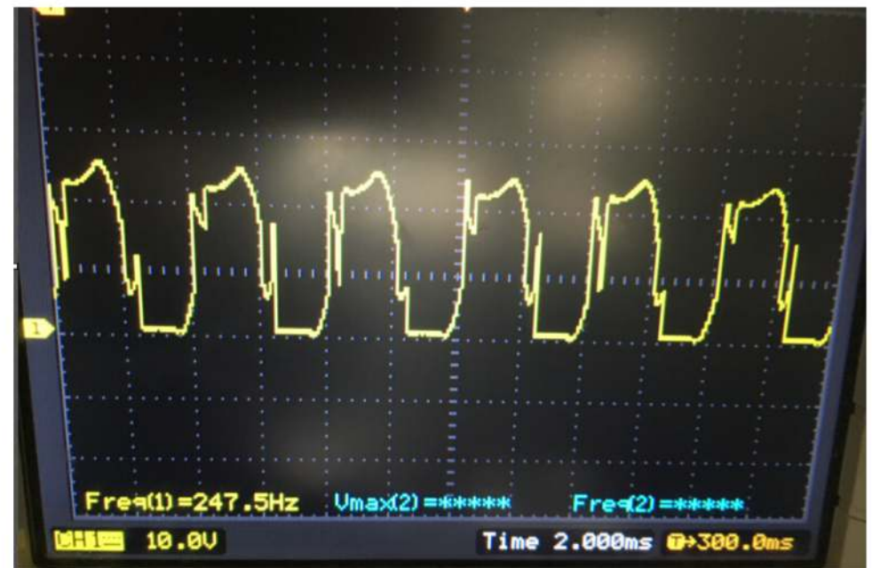
Figure 2: Pump's waveform under PWM modulation, but without customized PWM function
