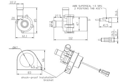
More application: roof air cooler, bus&yacht air conditioner, etc.. More billowy flow to 35 L/M and higher water head to 9 Meter TA60 pump is available, please freely contact us for detail!
